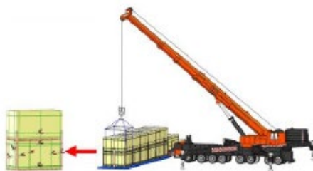
Vertical landscape package unloading with crane
