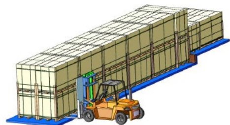
Vertical landscape package unloading with forklift
