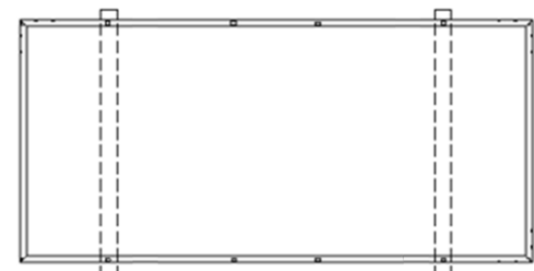
Figure 4: Bolt installation for 66 cell
