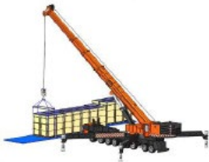
Vertical portrait package unloading with crane
