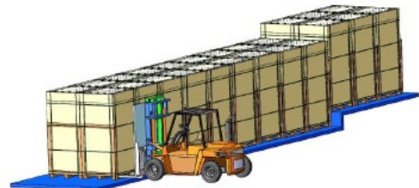
Vertical portrait package unloading with forklift
