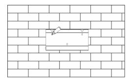
• Drill holes with electric drill, make sure the holes are at least 50mm deep, and then tighten the expansion tubes.
