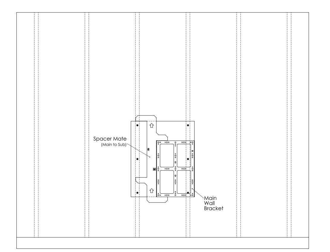
Slide the "Spacer Mate" into position making sure there is no play between the bracket and the "Spacer Mate".
