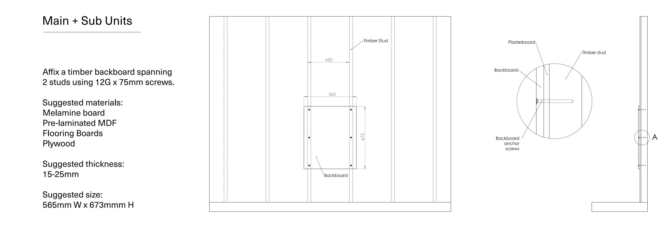
Install the wall bracket for the Main Unit using the 4 corners plus 2-4 more fixings to secure
