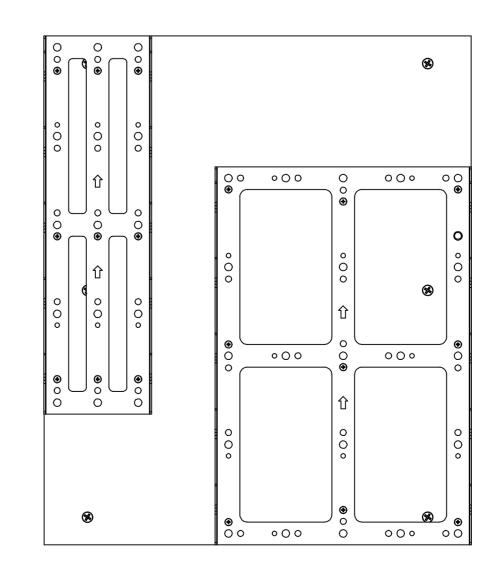
Once you have screwed in the brackets you may remove the "Spacer Mate" and mount the units on the brackets.
