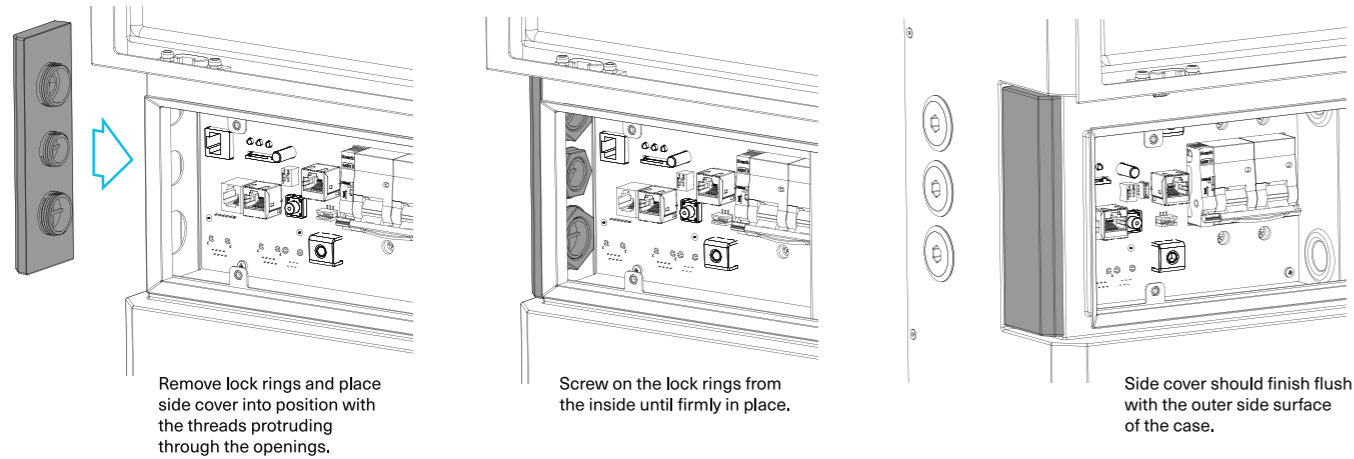
Fig. 35. Sealing the System
