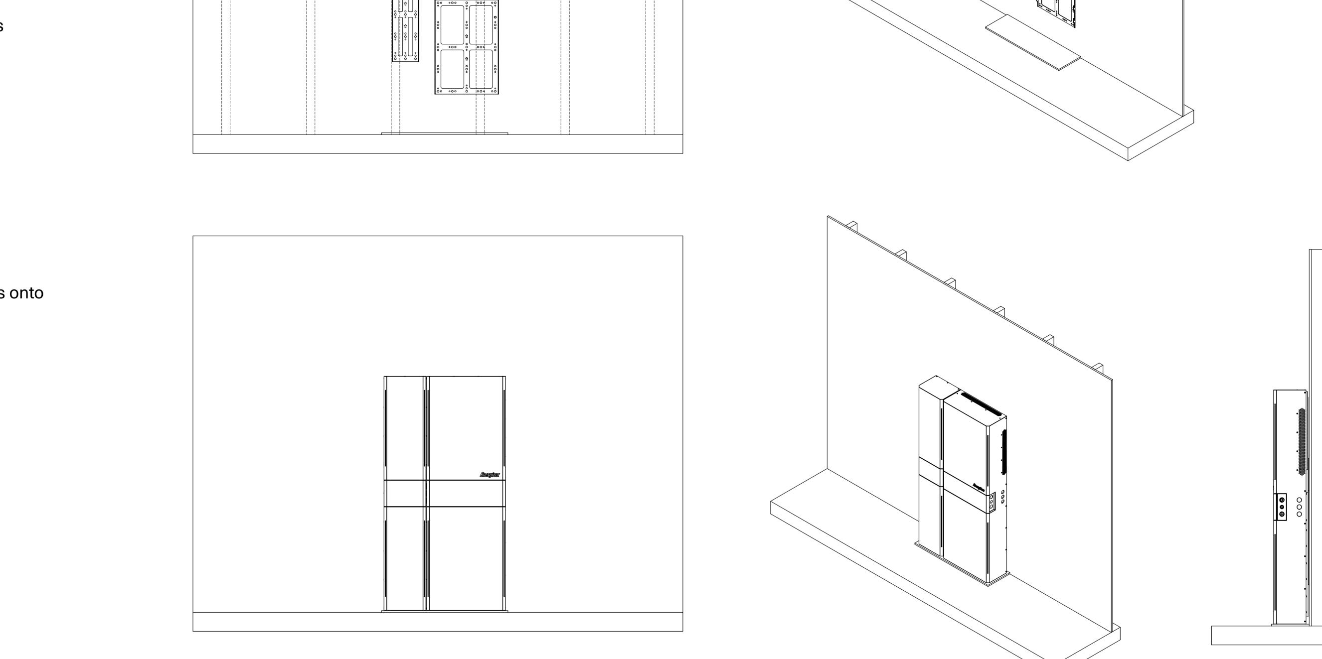
Carefully mount units onto wall brackets.
